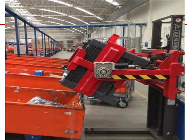
**CARRELLO ELEVATORE-RIBALTATORE DI CONTENITORI PER PICKING**
